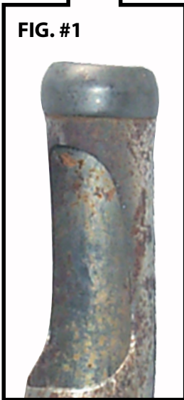
OEM conventional tine with normal wear in rocky turf
