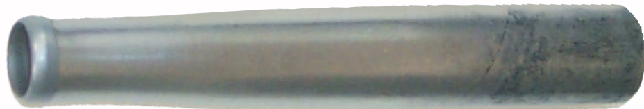
A JRM Dillennium™ tine with normal wear after 18 greens
