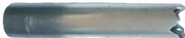
OEM conventional tine with normal wear in rocky turf
