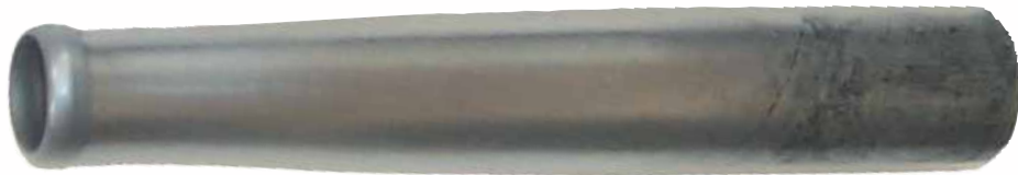
A JRM DILLENNIUM® tine with normal wear after 18 greens
