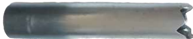
OEM conventional tine with normal wear in rocky turf
